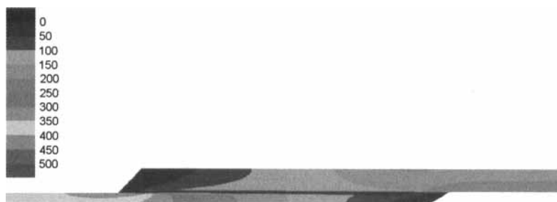
FIGURE 4 Maximum principal stress contours in overlap region. 22°C, unidirectional adherend, 20 kN load. (See Color Plate I).
