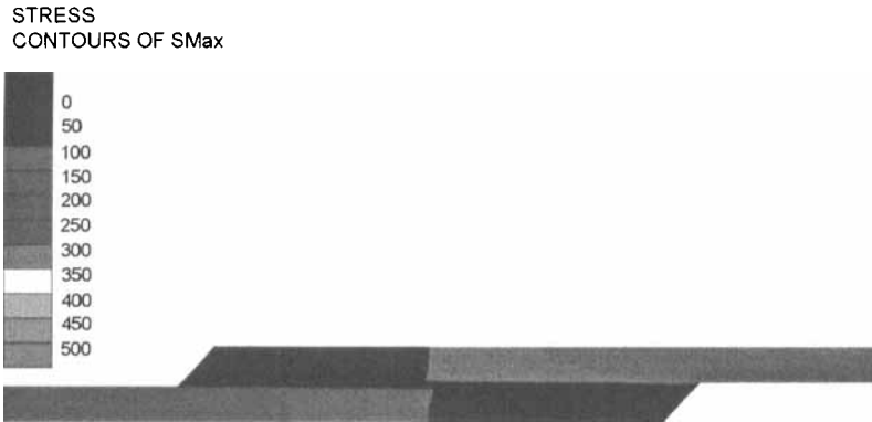
FIGURE 9 Maximum principal stress contours in overlap region. 22°C, multi-directional adherend, 20 kN load. (See Color Plate IV).
